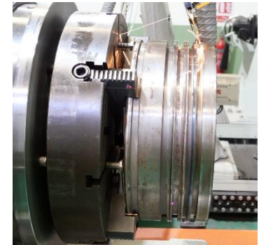
CLADDING OF PISTON RING GROOVE
