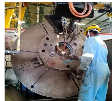
RECONDITIONING OF CYLINDER COVER
